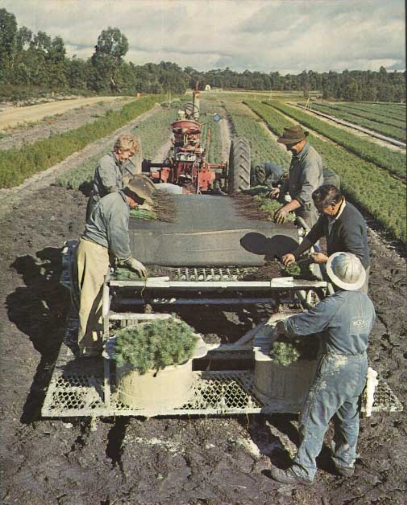
Pine seedling lifting unit operating at the Longford nursery of A.P.M. Australian Paper Manufacturers Ltd
