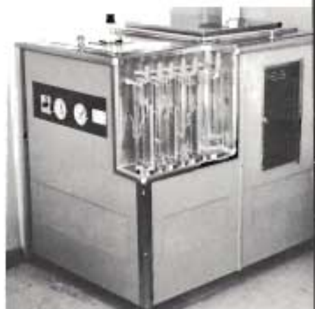
The protein sequencer — a machine developed in Melbourne to determine protein structures.
