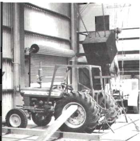
Impact testing of the protective frame on a tractor at the University of Melbourne's tractor testing station at Werribee.
